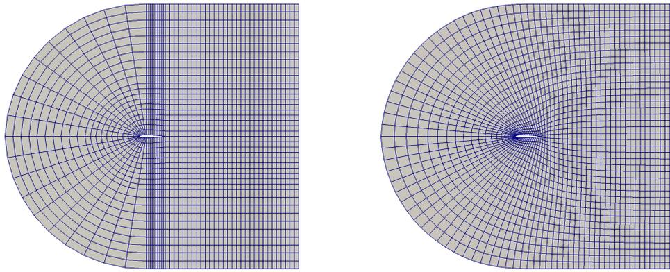
Figure 1: The initial mesh around the airfoil (left panel), and the converged optimized mesh (right panel). Notice the effect of the increased spring constant near the airfoil mesh boundary.
