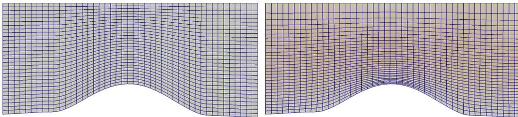
Figure 2: The initial mesh above an artificial hill (left panel), and the dynamically optimized mesh featuring inhomogeneous spring stiffness (right panel). Notice the resulting grading in the height direction.
