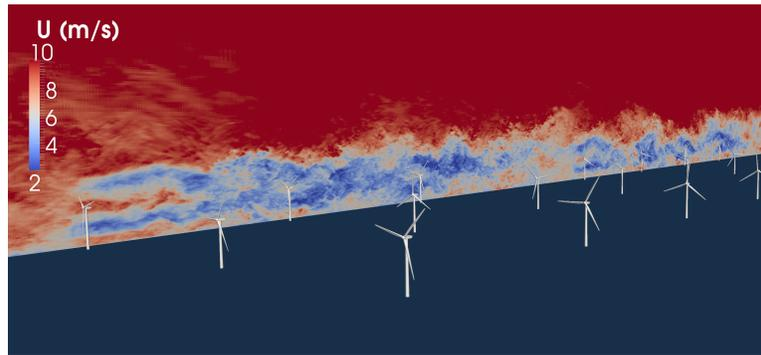
Figure 1: A vertical slice of instantaneous resolved wind speed in the Lillgrund offshore wind farm computed by Churchfield et al. [1]
